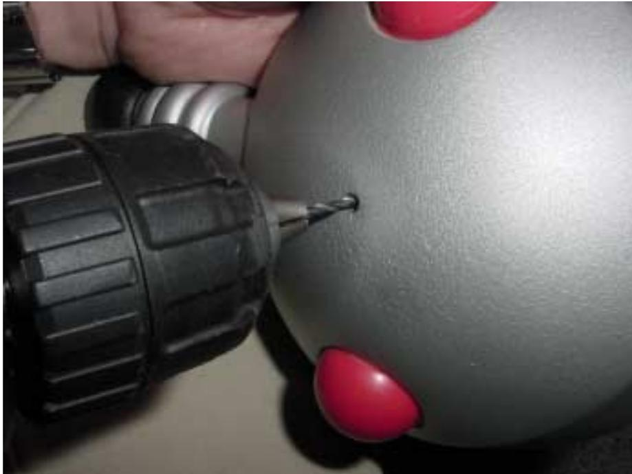
The centering of the eyepiece and head is accomplished by mounting a strip of machined steel to the underside of the head. Position the strip as shown with the edge of the steel  $\frac{1}{2}$ " from the edge of the head. Mark where the pilot hole you will be drilling will be with a pencil.
