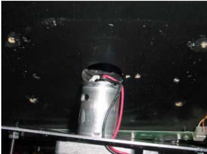
Push the mounting plate up so that it's flush and hold it in place.
