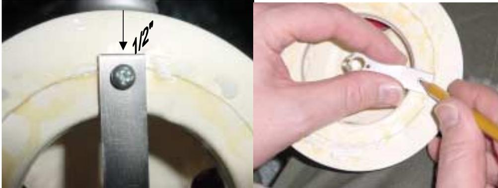
Drill a  $\frac{3}{32}$ " hole on your mark and secure the centering strip with one of the screws provided as shown. Your results should resemble the finished product below.
