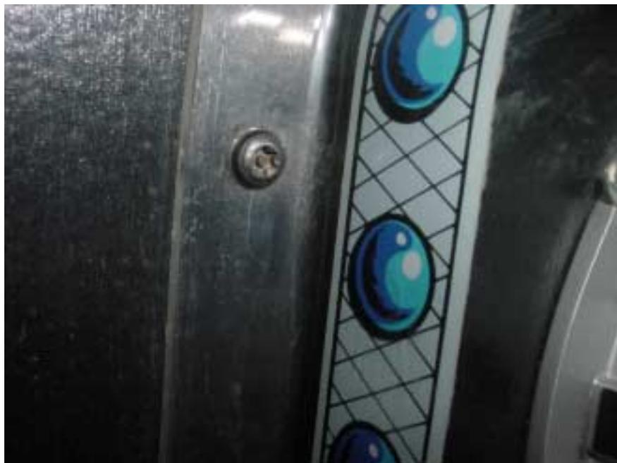
Remove the Dalek by removing the 4 ¼” Screws that are attaching it to the backbox. Keep the washers as we will be using them.
