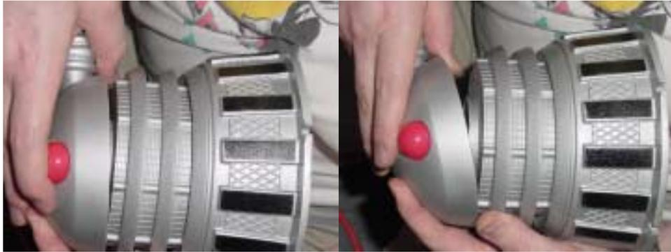
We will now adapt the head to be mounted on the assembly. Drill a 3/32" hole through the top of the head where the indent is.
