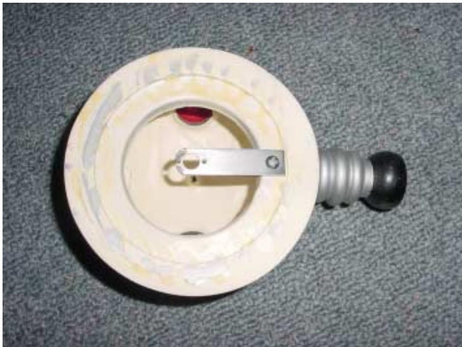
Mounting the head on the shaft is accomplished by putting the hole in the centering strip over the shaft and screwing the head down to the shaft from the top with the enclosed 6/32" allen head cap screw.
