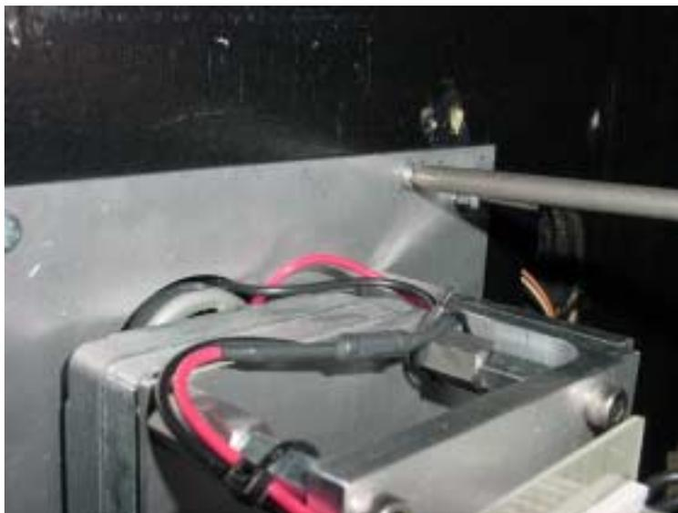
Connect the single large connector on the one end of the wiring harness to the Wobble Head circuit board and move the flasher bulb to the socket on Wobble Head. Raise the backbox of the game to the upright position.
